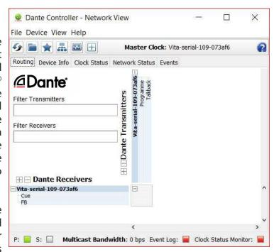
time network monitoring, including device-level latency and clock stability stats, multicast bandwidth usage, and customized event logging, enabling you to quickly identify and resolve any potential network issues. You can also quickly and easily backup, restore, move, and reuse Dante® network configurations using Presets, and edit Dante® routing configurations offline.
